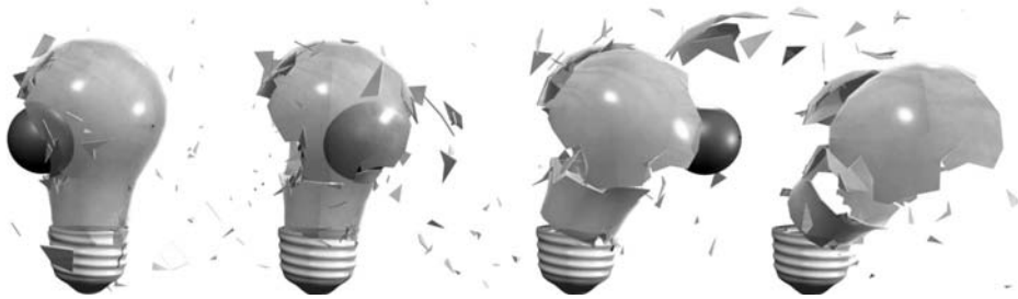
FIGURE 6. A measure of discrete strain is used to fracture a thin shell in this simulation of a shattering lightbulb.
